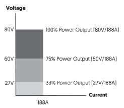
Using one autoranging PSU instead of several traditional DC sources saves both cost and bench space. Despite the units offering such a large output range, they are still incredibly power dense. 18kW of output power is provided from 3U of rackmounting height.
