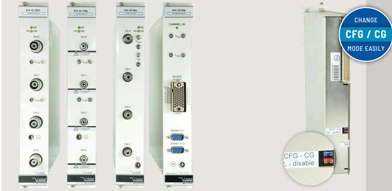
EHS modules are multichannel high voltage power supplies in MMS system (Eurocard format). With up to 32 channels each single channel has an independent voltage and current control. The module is made of high-precision components such as 24 bit ADC and up to 20 bit DAC and provides comprehensive safety features.
